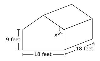
The base of the shed will be a square measuring 18 feet by 18 feet. The height of the rectangular sides will be 9 feet. The measure of the angle made by the roof with the side of the shed can vary and is labeled as  $x^{\circ}$ . Different roof angles create different surface areas of the roof. The surface area of the roof will determine the number of roofing shingles needed in constructing the shed. To meet drainage requirements, the roof angle must be at least 117°.
