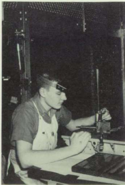
Inspecting Lathe Center with Sine-bar, indicator and Gage Blocks
